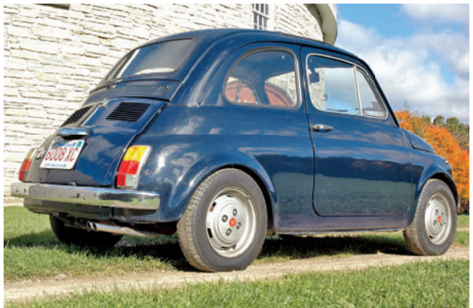
There's no shortage of replacement sheetmetal available to renew your rusted 500. The wheel arches, lower doors and the grille above the engine compartment are common places to find corrosion.
