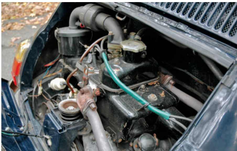
Fiat aircooled twins were never known for their power, but they are easy to work on (though the spark plugs can be tough to get out of their wells), and parts are still widely available.
